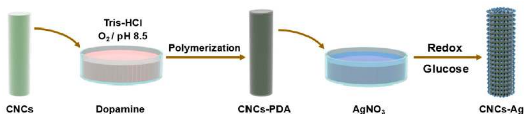
Figure 6. Synthetic route of nanocrystalline cellulose-silver (CNC-Ag) composite [110].
