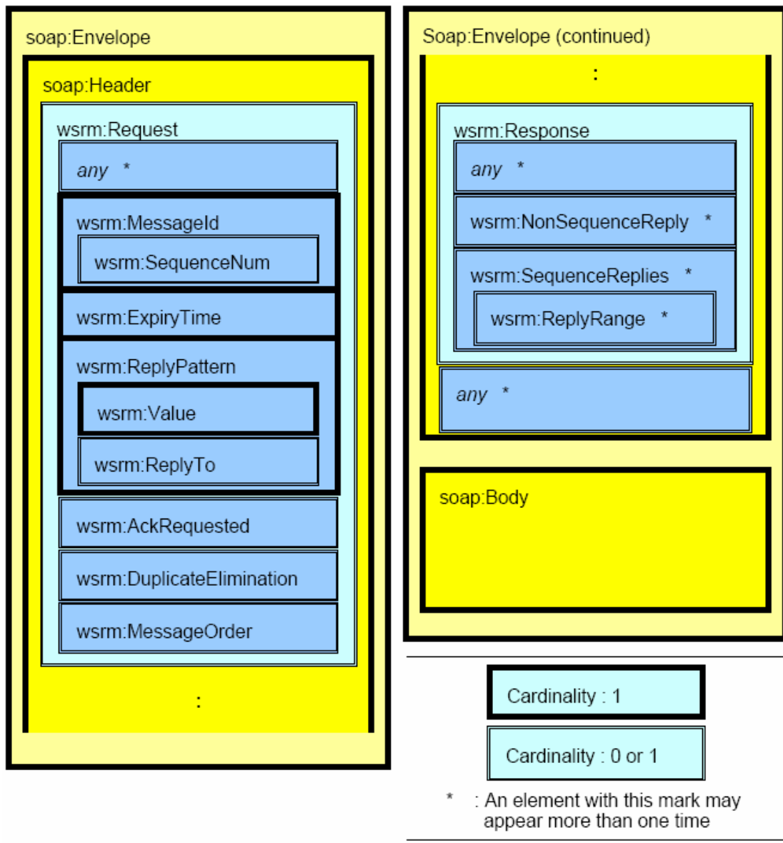
Figure 6-2 Structure of WS-Reliability elements
