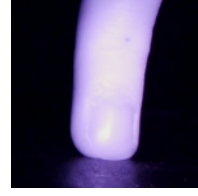
Figure 10: Diffusion of light source on finger as viewed by a camera. We have adjusted the exposure to ensure that the camera is not saturated.
