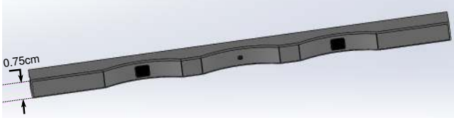
Figure 3: Concept-art of a product version of Okuli, to be fit into the edge of a small mobile device with a thickness around 7.5mm.
