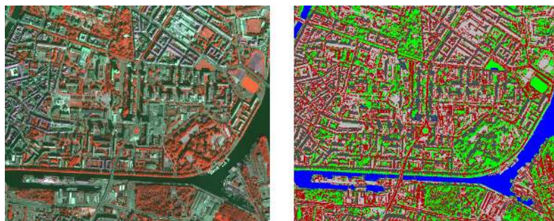
Fig. 4. Relevance of the 2-D size-spectrum local signature to classify pixels in multi-spectral remote sensed images: input (left) and classified (right) images.
