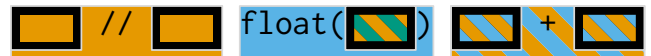
Fig. 2. Blocks for the integer division operator, the float function and the addition operator
