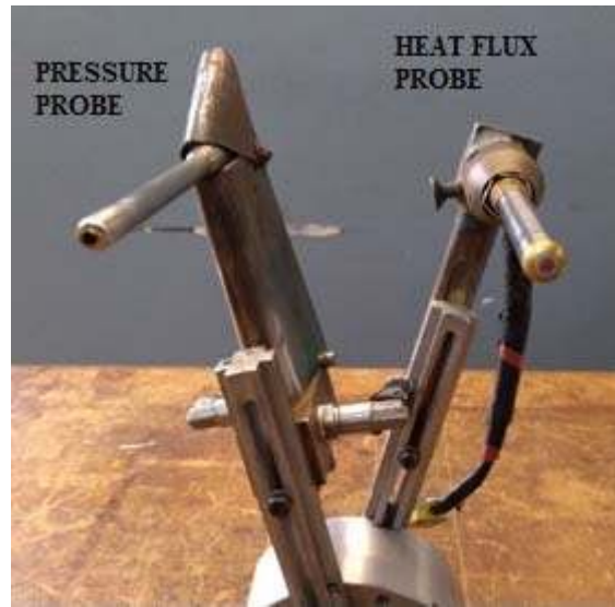
Figure 12. the probes used to apply the Heating Rate Method
