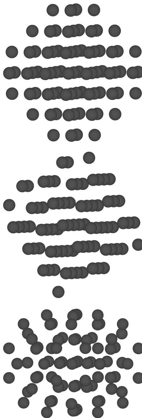
FIG. 9. The (a) fcc, (b) hcp, and (c) global minimum LJ-type structures of Ar_{79} for comparison.
