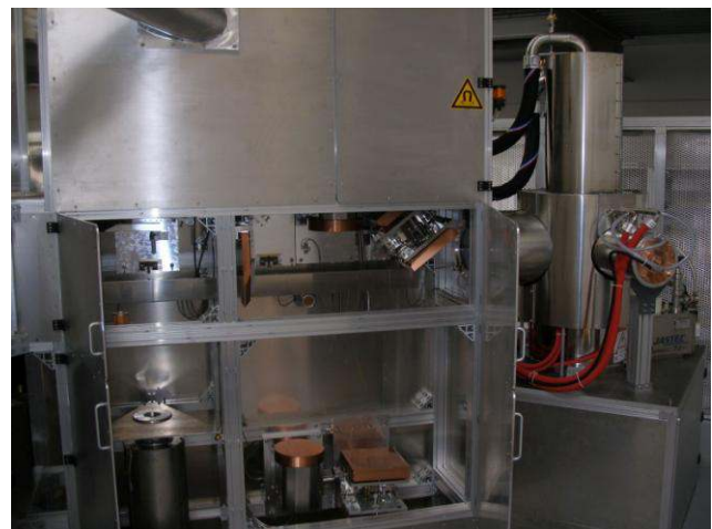
Fig. 2. Gyrotron (right) connected to a Matching Optics Unit (left)
