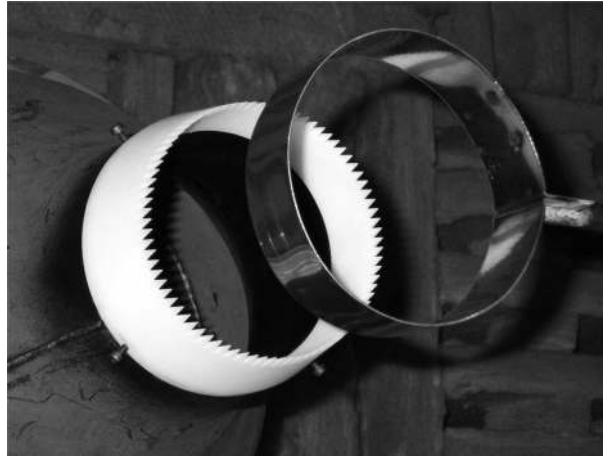
Figure 7: The jet-ring arrangement as an alternative experimental setup for studying turbulence-interaction noise from an airfoil in circular geometry, from [20]. The serrations on the nozzle suppress the acoustic back-reaction from the ring, which would induce self-sustained oscillations involving the jet instability modes.
