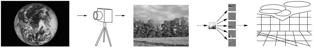
Figure 2.1: Problem setting. From left to right: Particle system known as the world. Observation device in the world (and part of the world). Image produced by the observation device. Low-level analysis of the image, taking advantage of image statistics. Image understanding, i.e. extracting information relevant to the observer from the image.
