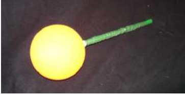
Figure 2: The marker object that is tracked through the scene to establish 2D correspondences between camera frames consists of a bright orange ball on a stick.
