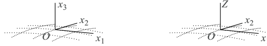
FIGURE 3. Local coordinate systems used in flamelet modeling. Point O is fixed on the stoichiometric surface.
