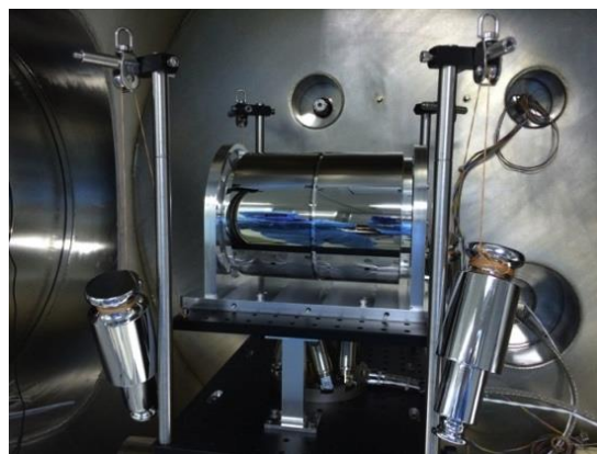
Figure 2. Left Panel: the effective area (single unit) of the current design of the eXTP SFA optics. On the right panel the very first prototype, successfully integrated at IPOE (Tongji University), is shown. The prototype has successfully passed vibration (5-6 g) and shock (5g) tests and its first performance testing session.
