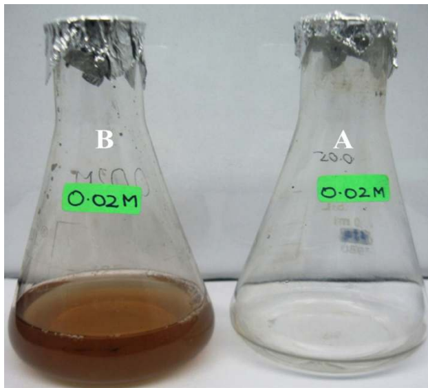
Fig. 3 Biosynthesis of silver nanoparticles—colour change reaction: conical flasks containing the extracellular filtrate of the Streptomyces sp. (09 PBT 005) biomass (a) and conical flasks are containing the extracellular filtrate of the Streptomyces sp. (09 PBT 005) biomass after exposure to \text{AgNO}_3 solution (b)
