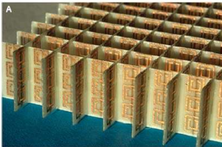
Figure 3. A Negative Index Metamaterial Formed by SRRs and Wires Deposited on Opposite Sides of a Standard Circuit Board. (From Ref. [14])
