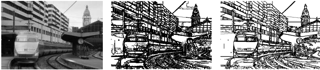
Figure 2: Maximal meaningful boundaries. 1. Original image, 83,759 level lines 2. All meaningful boundaries: 11,505 detections. 3. Maximal meaningful boundaries. Only 883 boundaries remain, while the visual loss is very weak.
