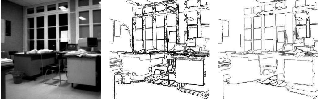
Figure 14: Regularity detectability. The original is the left most. In middle, we display the 204 detected contrasted smooth boundaries as defined in Def. 4. On the right, the 96 smooth boundaries, with no contrast information, defined in (20). All the main boundaries are already present. Of course, contrast may be the main cause of small NFA, since regularity acts at larger scales. For instance, the window panes have NFA about 10^{-150} with contrast and 10^{-15} with regularity only (which still make them detectable in any image database). The desk on the bottom right has a NFA equal to 10^{-60} with contrast and 10^{-20} with regularity, which is already very small.
