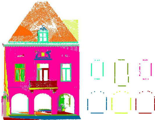
Figure 5. An example showing holes in the wall recognized as windows.
