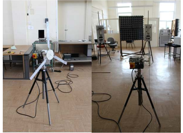
Fig. 5. Photos of the experimental setup. The CW radar was facing the rotating windmill like target.
