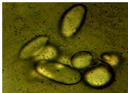
Plate 1: Optical micrographs of Bintasuga showing starch granular shapes at \times 1000 magnification.
