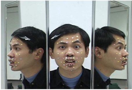
Figure 1: The image data captured by DV camera (resolution 720x480). 54 markers are placed on the subject's face and lips.
