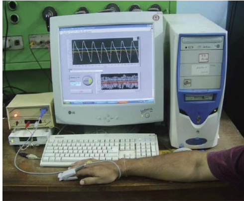
Figure 3.2 Developed analog front-end for PPG acquisition
