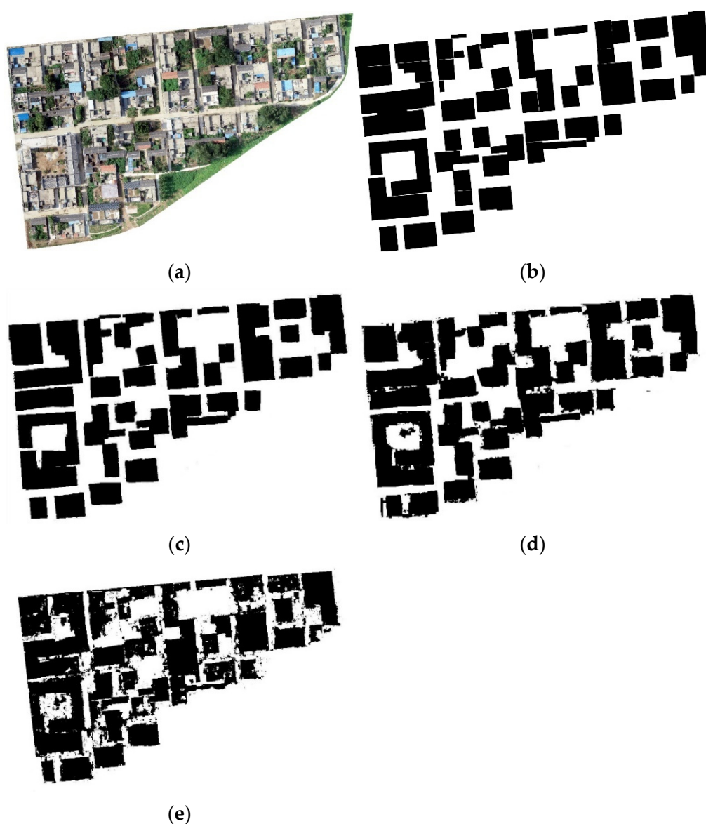
Figure 12. The original images, the results of the field investigation and the extraction results of different methods in Sanniangmiao Village, respectively: (a) original image; (b) results of field investigation; (c) extraction results of CDD-Net; (d) extraction results of ResNet + ASPP; (e) extraction results of ResNet + UNet.
