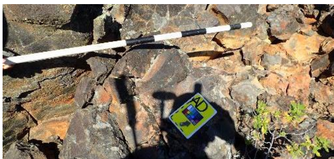
Figure 8. Temporary tags used to mark candidate sample locations; tags included an alphanumeric label, color bar, scale bar, and rotatable north arrow
