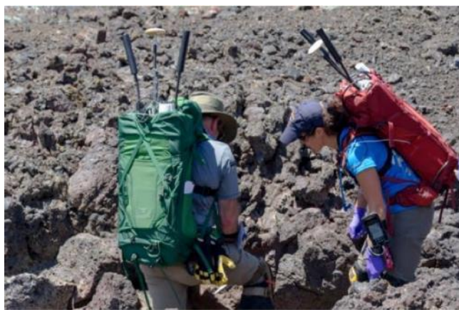
Figure 3. BASALT-1 EV crewmembers in the field wearing the informatics backpacks and wrist displays
