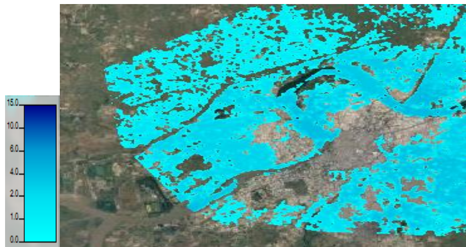
Fig 7: Flood Inundation map for predicted image for the year 2015.
