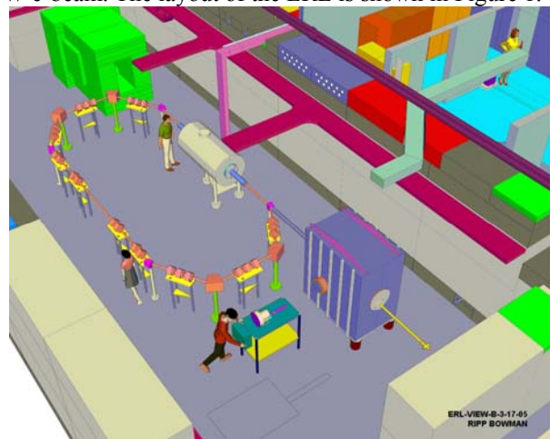
Figure 1: Layout of ERL. The gun is the square structure (blue) on the right, followed by the round 5-cell cavity cryomodule and the beam dump shielding.
