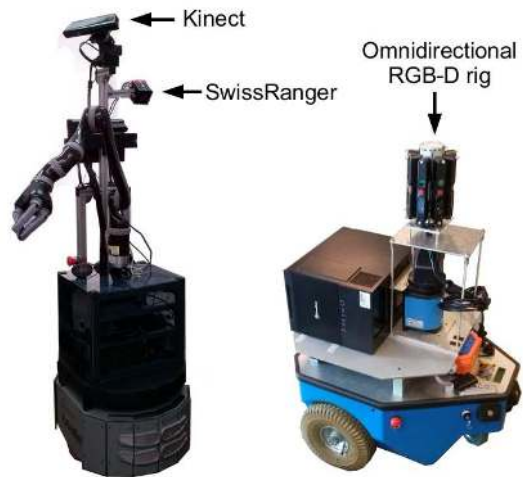
Fig. 4. Robots which mount rigs of range and RGB-D cameras.
