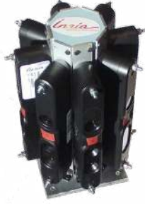
Fig. 5. Omnidirectional RGB-D camera rig.
