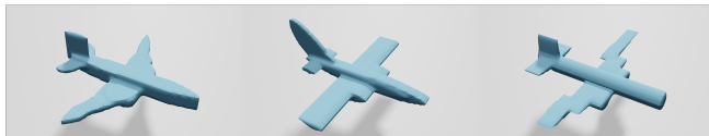
Fig. J. Reconstruction results by setting constraints on the extrusion plane orientation. Left: Top Extrude. Middle: Side Extrude. Right: Front Extrude.
