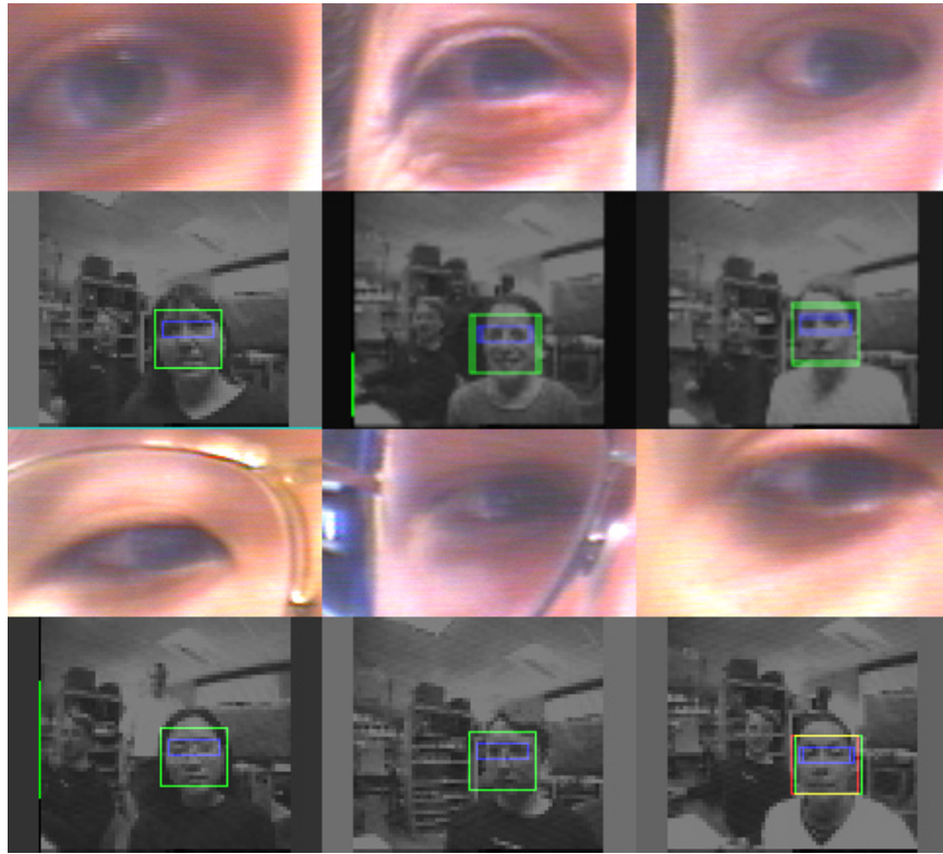
Figure 6: Six detected faces and eyes. The lower image of each pair shows the post-saccade location of the detected face. The upper image of each pair shows the section of the foveal image obtained from mapping the peripheral template location to the foveal coordinates. Only faces of a single scale (roughly within four feet of the robot) are shown here.
