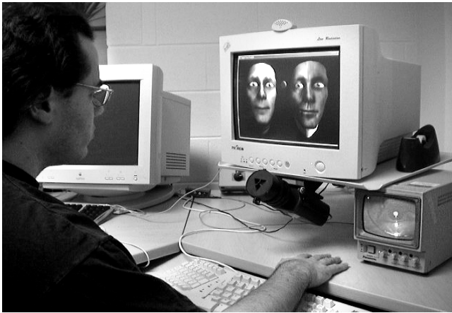
Figure 4. User interacting with FRED. An eye tracker camera mounted below the computer screen is used to determine which agent the user gazes at.
