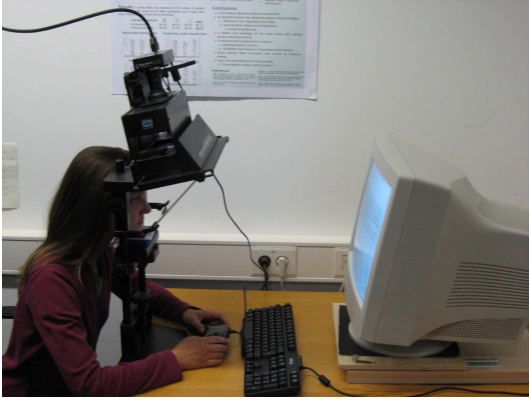
Fig. 1 Experimental setup. Participants sat comfortably in a chair and watched the movies on a computer screen. Head stability was achieved by means of a chin rest.
