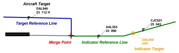
**Figure 2. Depiction of a Generic Relative Position Indicator (RPI) Application.** The indicator target of the aircraft on the Target Reference Line is depicted the same distance away from merge point along the Indicator Reference Line, accounting for turn anticipation through the route segment transition.
