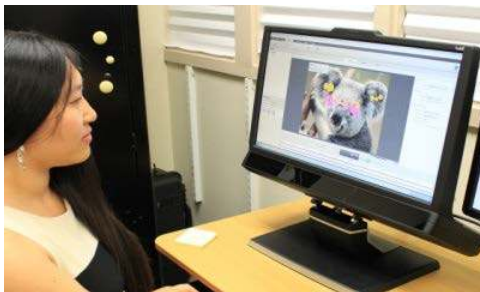
a. Eye tracker with removable monitor
