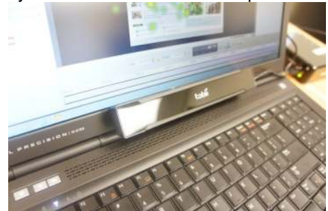
c. Eye tracker attached to a laptop screen
