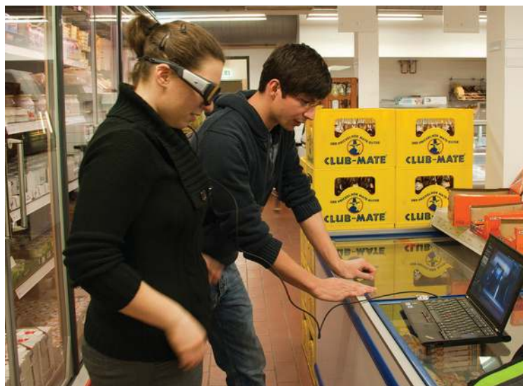
Figure 1. Mobile eye tracking in a supermarket scenario. The person in the front is wearing glasses with integrated mobile eye tracking. In this consumer study, the participants' eye movements are recorded when they perform shopping tasks. The picture was taken as part of a research project on mobile, unconstrained eye tracking.
