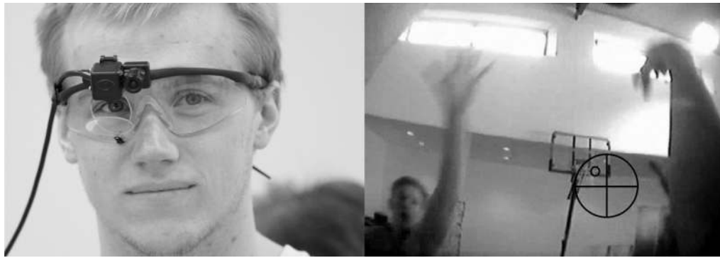
FIGURE 1 | Participant wearing an Applied Science Laboratories (ASL; Bedford, MA) mobile eye-tracker ( Left ; monocular set-up with a scene camera and an eye camera capturing eye movements via a mirror in front of the participant's right eye) and an exemplary image captured by the scene camera with the circle indicating the current gaze position ( Right ; the cross hairs denoting the detection of the pupil) (left picture © Ledchumanasarma).
