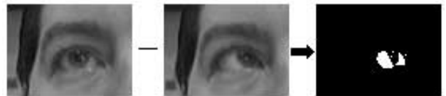
Figure 2: Motion detected by frame differencing is thresholded and used as a mask for the left-right image differencing.
