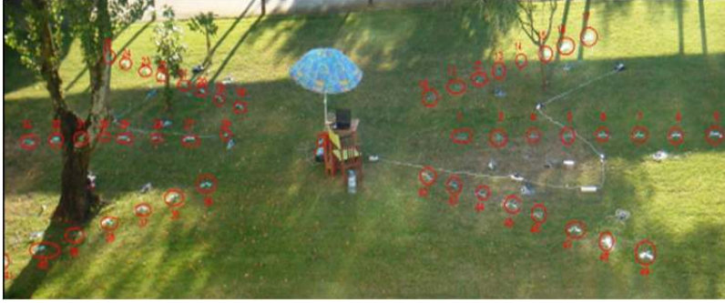
Fig. 3. Nodes distribution according the circular topology, at an outdoor environment
