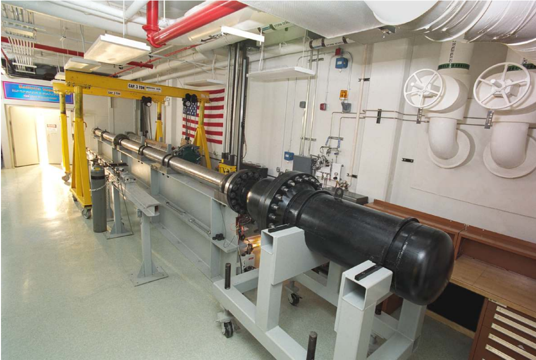
Figure 3. Gas Gun Used for Ballistic Impact Testing
