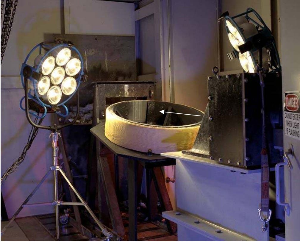
Figure 1. Fabric Specimen Wrapped Around Ring Fixture. Arrow Shows the Location of Impact.
