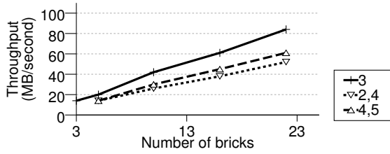
Figure 11: Aggregate throughput of FAB clusters with the DB workload. “3” means three-way replication, “2,4” means 2,4 erasure coding.
