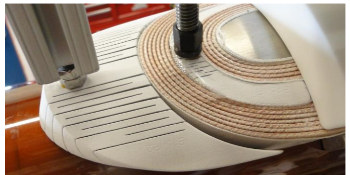
Fig. 1. Picture of ‘accordion style’ end parts first employed in LHQ. The end parts are plasma coated with alumina at 250 μm thickness for additional electrical integrity. The added flexibility accommodates the tendency for cable to separate from the winding mandrel surface also called cable spring-back. The inner end part tightly conforms to cable shape and the outer end part will easily conform to the inner turns after the addition of subsequent tooling and turns.
