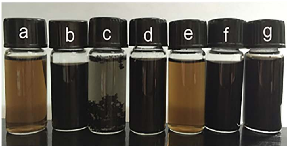
Fig 1. Photograph of the samples ( 0.1 \text{ mg}\cdot\text{mL}^{-1} , GO (a) and RGOs (L-AA RGO-1 (b), L-AA RGO-2 (c), D-GLC RGO-1 (d), D-GLC RGO-2 (e), N RGO (f), and TP RGO (g)).
