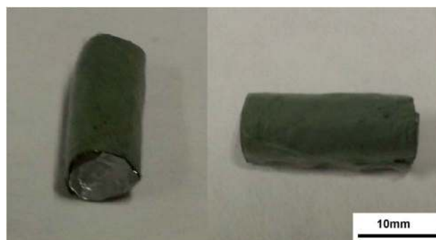
Fig. 7 Photos of PLLA/PANI/TSA2.4 fiber tube.
