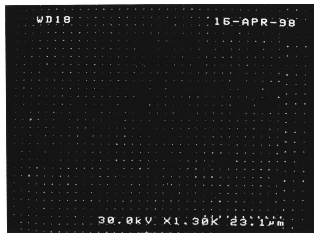
FIG. 3. SEM image of an electroplated Ni dot array of 100 nm diameter and 2.5 \mu\text{m} spacing embedded in an \text{Al}_2\text{O}_3/\text{GaAs} substrate.
