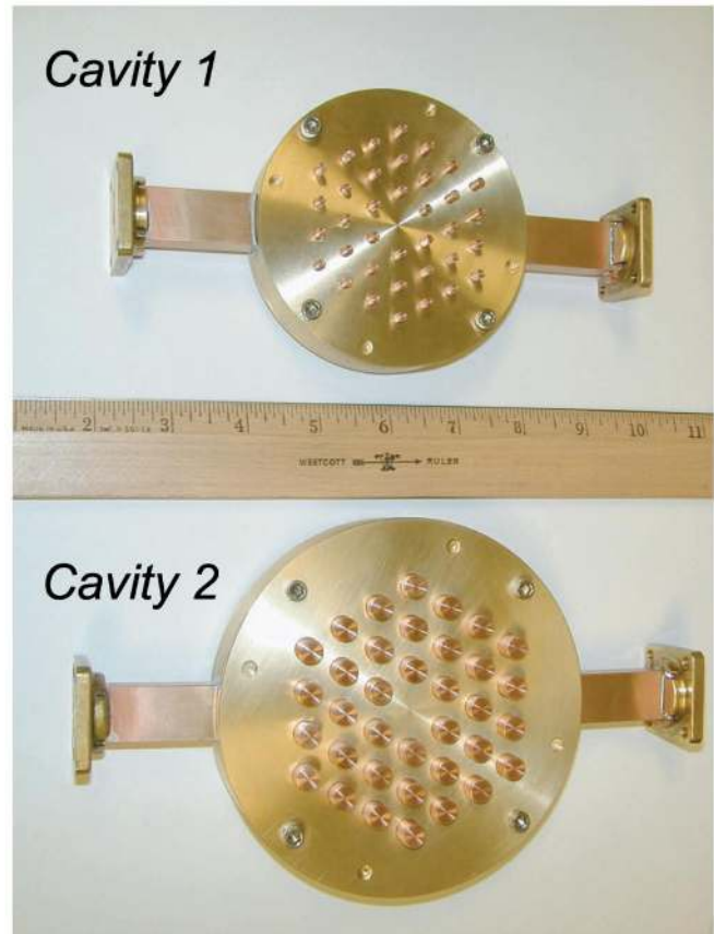
FIG. 4. (Color) PBG resonators built for the cold test.
