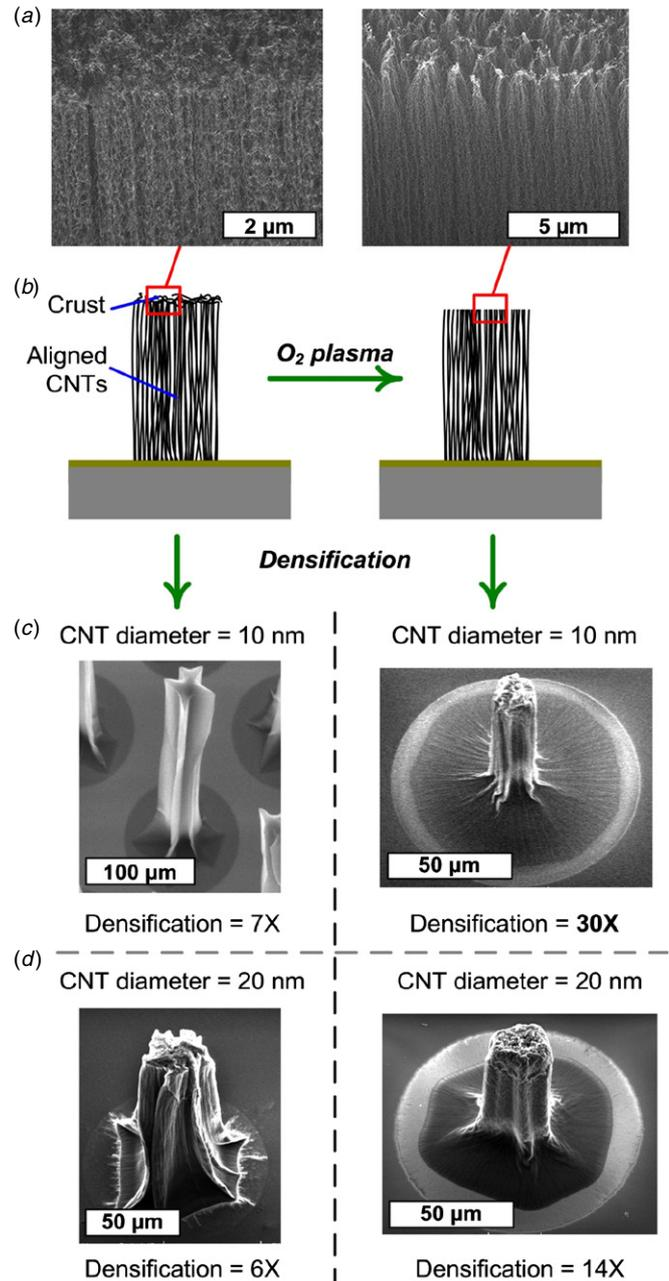
**Figure 6.** Influence of plasma etching and CNT diameter on the densification of cylindrical micropillars, using acetone: (a) SEM image of the crust layer on top of an as-grown micropillar; (b) schematic of micropillars as-grown and after plasma etching which removes the crust; (c) SEM images of micropillars after densification, with CNT diameter 10 nm; and (d) SEM images of micropillars after densification, with CNT diameter 20 nm.
