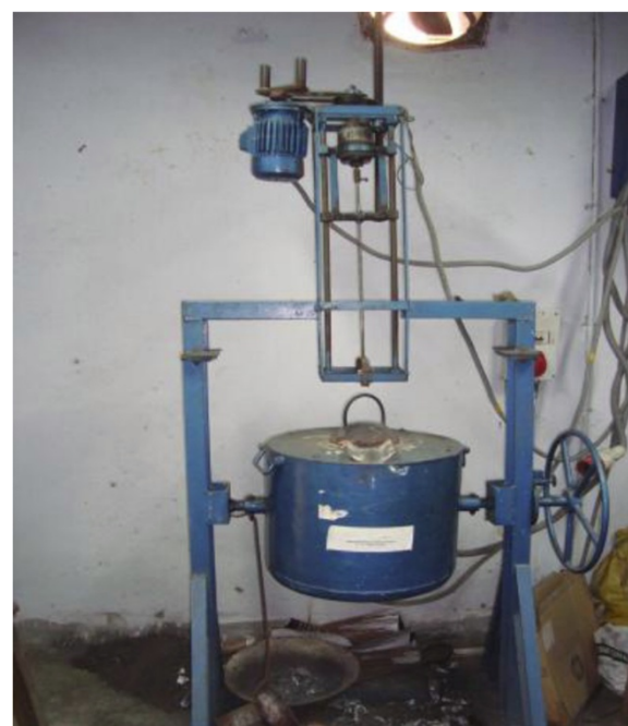
Figure 6 Electric resistance furnace with stirring system (Behera et al. 2012).
