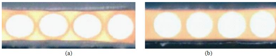
Fig. 2. (a) W-shaped and (b) previously obtained GI-PPOW illuminated by a Halogen-Tungsten lamp.
