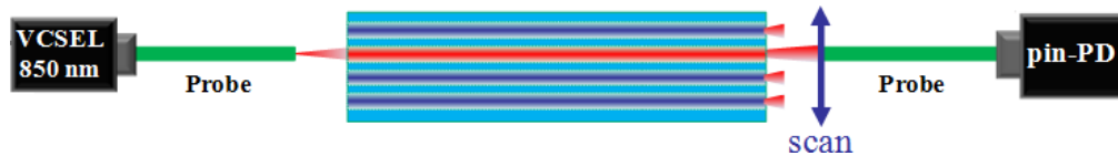
Fig. 6. Experiment setup for inter-channel crosstalk measurement.
