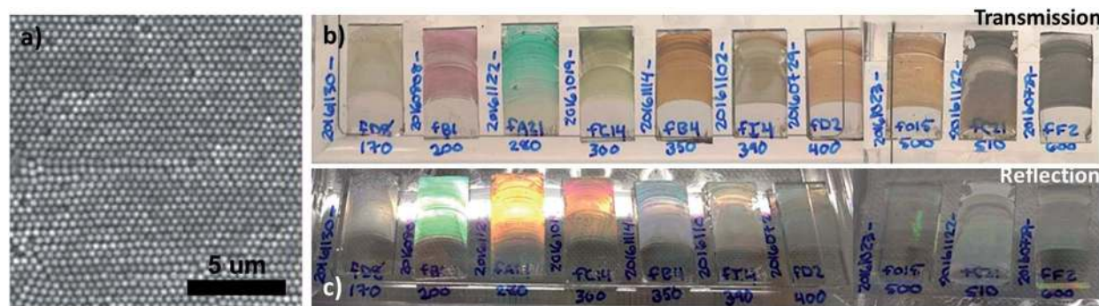
Fig. 1 (a) SEM image of a 500 nm PS bead film, (b) transmission and (c) reflection camera images of the PS templates showing film uniformity over a >1 \text{ cm}^2 area. PS templates reported in (b) and (c) are 1 \times 2 \text{ cm}^2 .
