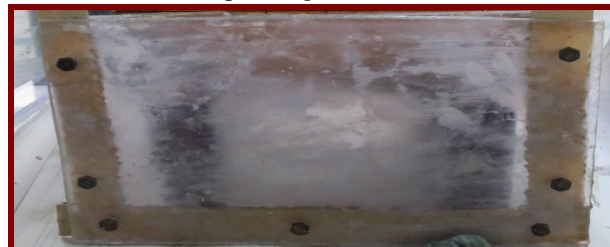
Fig.4 Mould for plate casting
