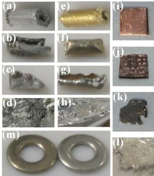
Figure 15. (a) Non-exposed aluminium sample, exposed aluminium sample for (b) 15 min at room temperature, (c) 5 min at 100 °C, (d) completely dissolved aluminium at room temperature for 30 min (e) Non-exposed brass sample, (f) exposed brass sample for 5 min at 100 °C, (g) exposed brass sample for 2 h at 230 °C (h) completely dissolved brass for 3 h at 230 °C (i) Non-exposed Cu sample, (j) exposed Cu sample for 15 min at 100 °C, (k) exposed Cu sample for 30 min at 230 °C, (l) completely corroded Cu sample after 1 h at 230 °C and (m) non-exposed 316-stainless steel washer (right) & exposed washer (left) for 5 h at 230 °C.
