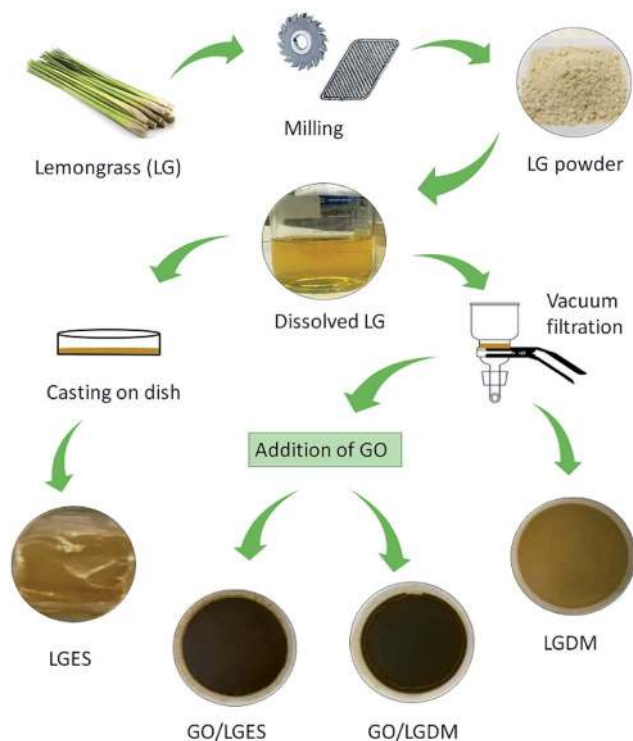
Fig. 10 Schematic fabrication process from lemongrass (LG) plant to membranes.
